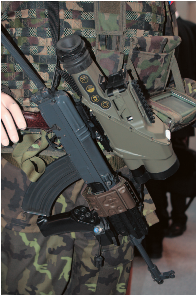
Weapon control attachment on EADS/Sagem Warrior21 ensemble.
